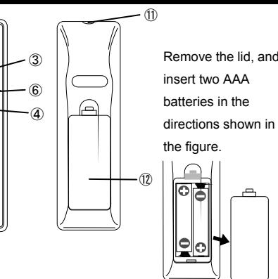
Remove the lid, and insert two AAA batteries in the directions shown in the figure.
